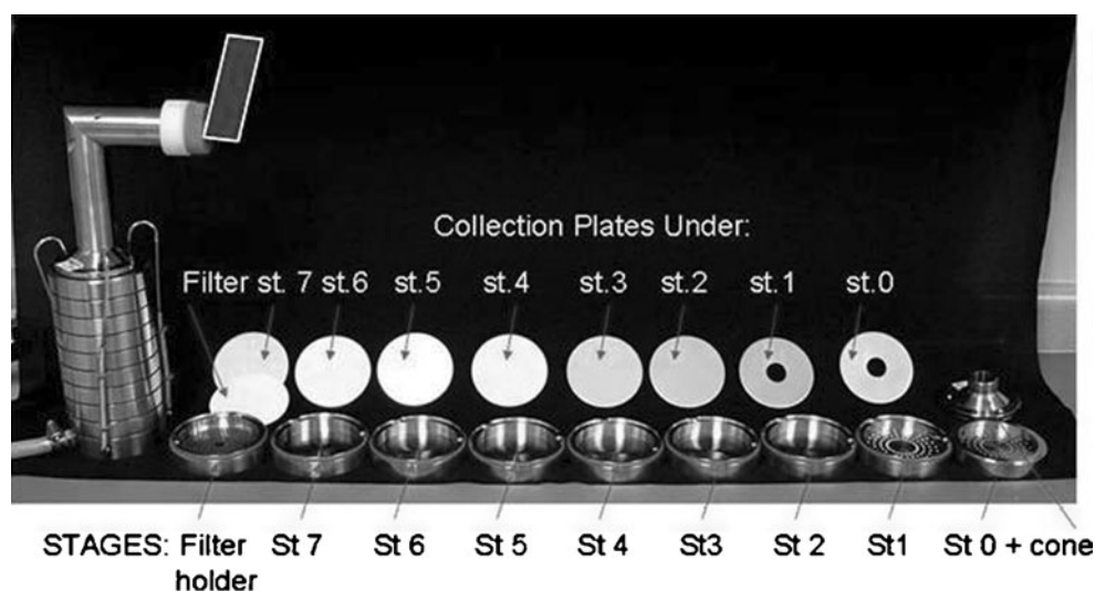
Fig. 1. Configuration of the full resolution Andersen 8-stage cascade impactor (ACI) (benchmark system)
